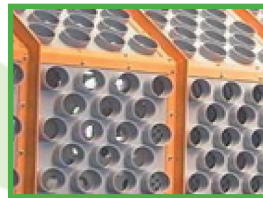
Screening plate with anti-wrap tubes
